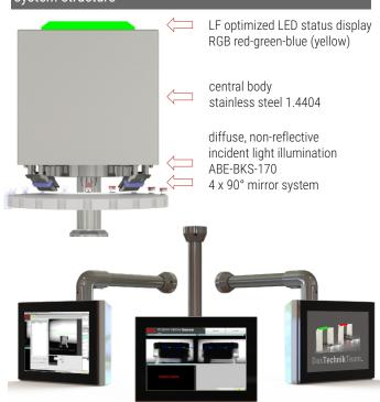
HMI housing stainless steel according to customer specification
